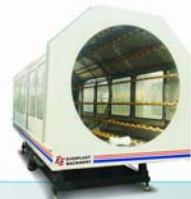
▲ 1200MM WATER COOLING TANK
